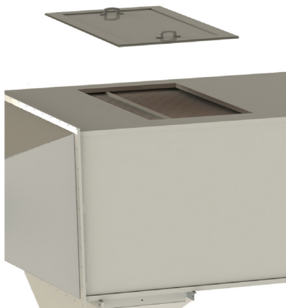
A lid can be lifted to clean the internals
